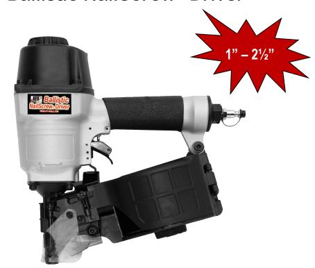
The NSDCN64 is a  $2\frac{1}{2}$ " (65 mm) Coil Nailer designed for high speed operation. It is well-balanced and powerful for heavy duty applications. It has a magnesium housing that is light weight. The magazine is tough nylon and easy to load. The flat angle magazine allows toe-nailing. The high durability driver blade and bumper are specially designed for long life.
