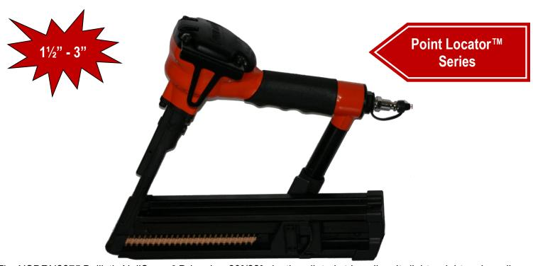
The NSDRN2275 Ballistic NailScrew® Driver is a 20°/22° plastic collated strip nailer. Its light weight and smaller size makes it perfect to maneuver and access tight areas. The NailScrew® point protrudes so it is easy to align. It has a rear load magazine with load and cock operation. It includes the case, fitting, wrenches, and oil.
