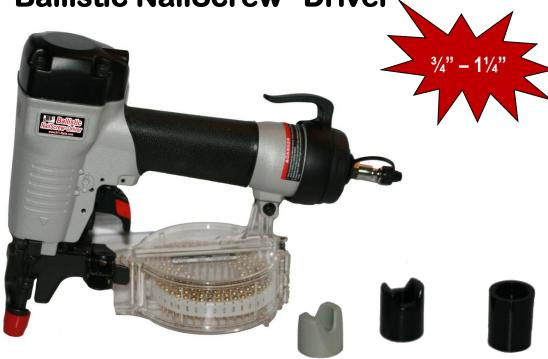
The NSDCN32 Ballistic NailScrew® Driver comes with four no-mar tips and a 360° rotating nose piece. This lightweight tool has an ergonomically designed handle for ease of operation and comfort. Features of this durable, powerful nailer include a sequential fire or bump fire switch on the trigger, an adjustable depth of drive, and a clear, see-through magazine.
